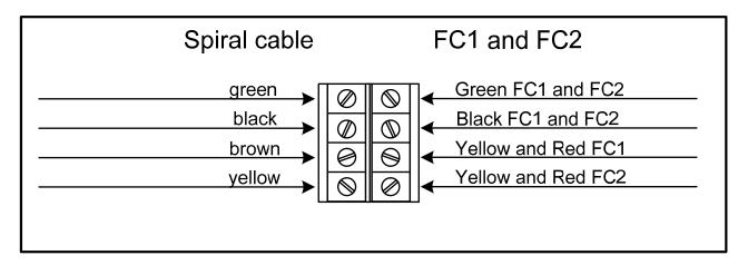
Connect the spiral cable to the AS130 (the card ASO13 is required)
