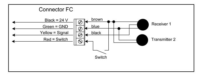
The switch closes if the FC starts to rotate!
